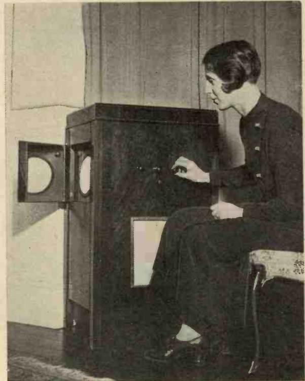
The arrangement allows of the image being viewed in a mirror at the side of the cabinet or directly, as may be preferred.
