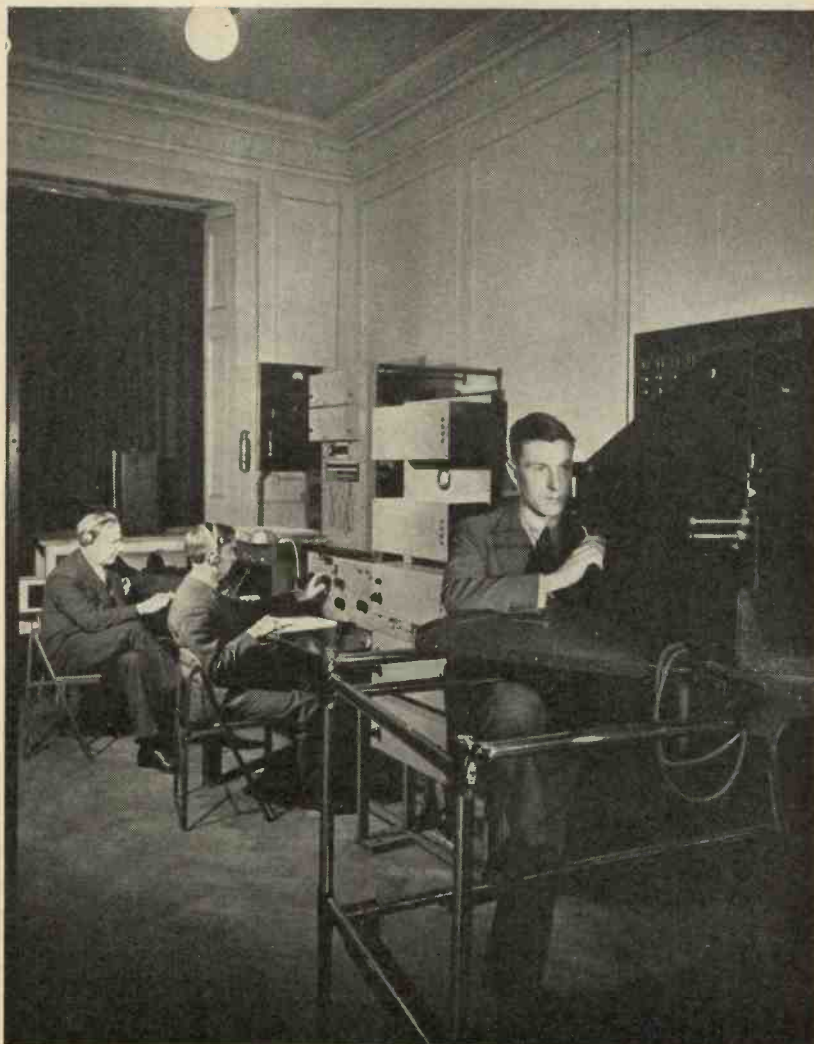
A scene during an actual 30-line television transmission. The projector (seen on the right) is mounted on rails and can be swivelled round to follow the movements of the artists.
