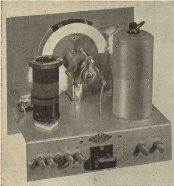
This photograph shows the rear of the signal booster which, as will be seen, is quite simple to build.
